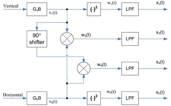
Fig. 2. Signal-flow diagram for a correlating polarimetric microwave radiometer.
