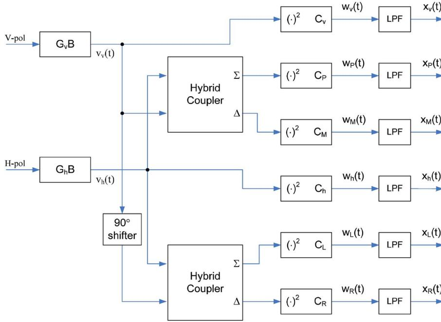
Fig. 1. Signal-flow diagram for a hybrid combining polarimetric microwave radiometer. Subscripts  $v$ ,  $h$ ,  $P$ ,  $M$ ,  $L$ , and  $R$  designate the vertical, horizontal,  $\pm 45^\circ$  slant linear, and left- and right-hand circular polarization channels, respectively.
