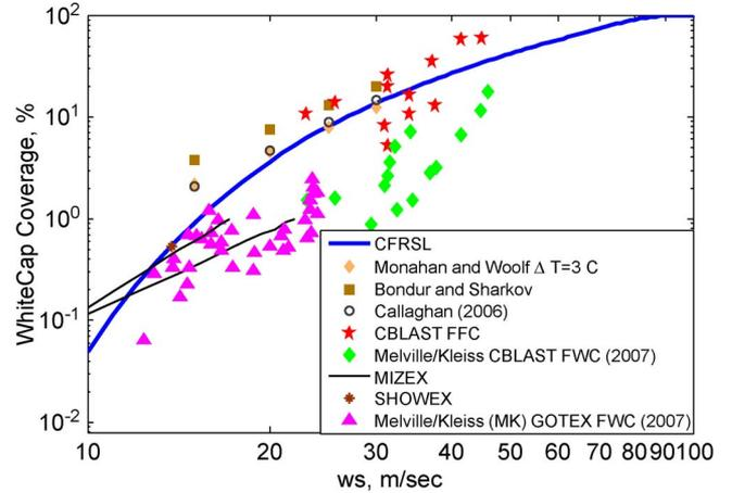
Fig. 1. CFRSL  $FF$  parameterization with respect to (solid curve) 10-m oceanic wind speed with empirical observations of percentage of sea foam coverage.
