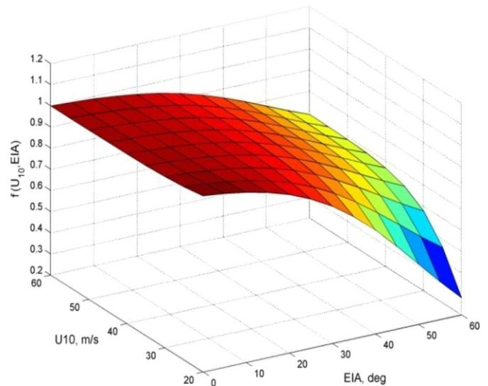
Fig. 2. Foam emissivity dependence [ $f(U_{10}, EIA)$ ] with respect to  $U_{10}$  (in meters per second) and  $EIA$  (in degrees) for H-pol.
