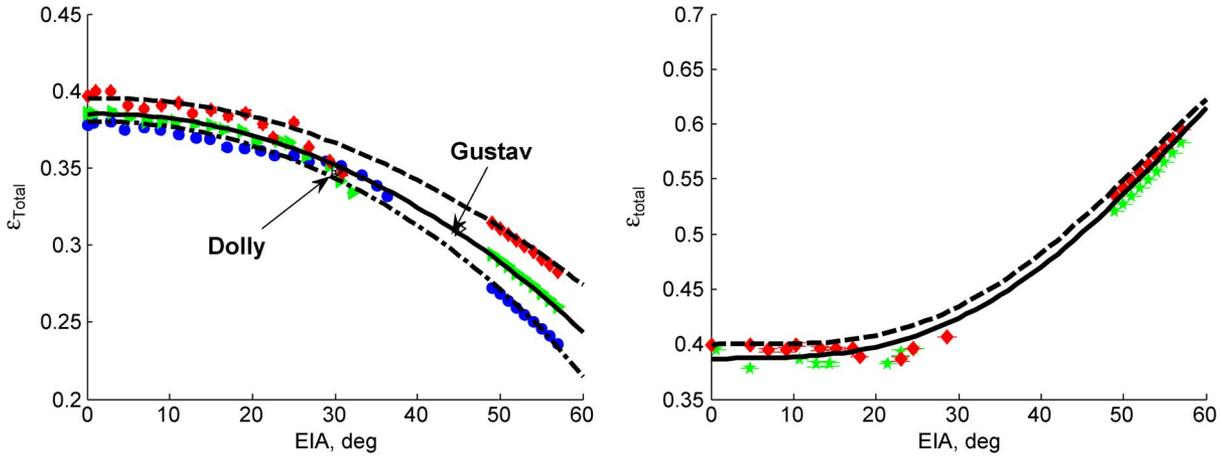
Fig. 3. Total ocean emissivity for (left) H-pol and (right) V-pol for wind speed bins of (○) (5–10 m/s), (\* and ►) (10–15 m/s), and (◊) (15–20 m/s), where the vertical bars represent one-standard deviation of the binned average.
