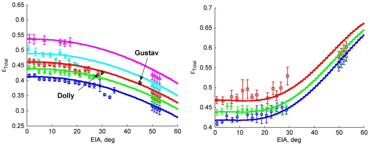
Fig. 4. Total ocean emissivity (left) H-pol and (right) V-pol for wind speed bins of (○) (20–25 m/s), (◊) (25–30 m/s), (◻ and ►) (30–35 m/s), (\*) (35–40 m/s), and ▲ (40–45 m/s), where the vertical bars represent one standard deviation of the binned average.
