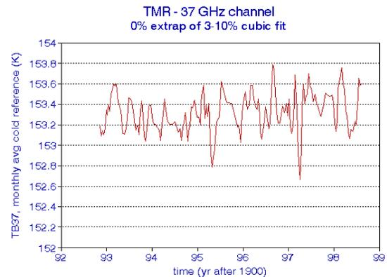
Figure 2. Time series of coldest TB at 37 GHz for the TOPEX Microwave Radiometer.
