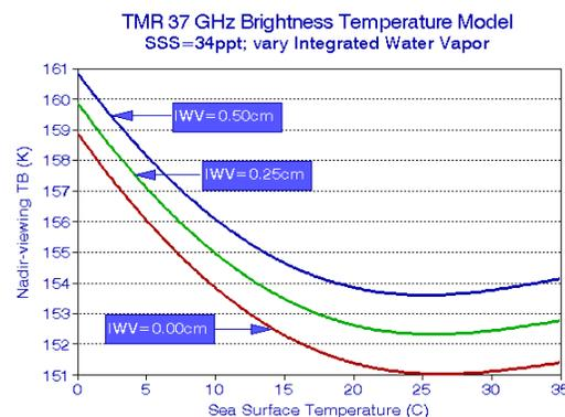
Figure 1. Modeled minimum TB at 37 GHz, nadir incidence angle.
