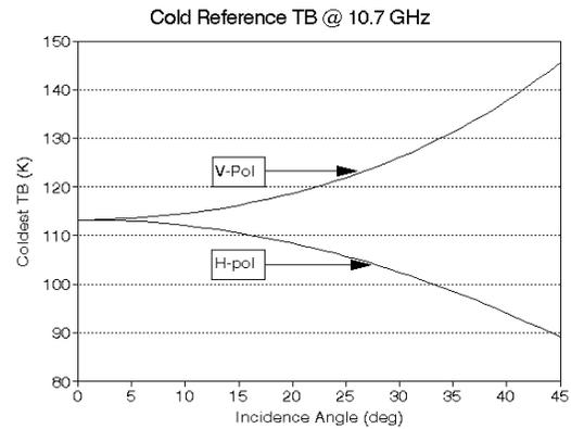
Figure 4. Cold reference TB at 10.7 GHz H- and V-pol versus incidence angle
