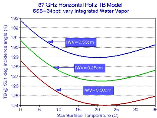
Figure 3. Modeled coldest TB at 37GHz, H-pol, 53.1deg incidence angle.
