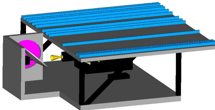
Figure 2. Conceptual drawing of constellation radiometer sensor.
