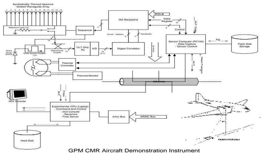
Figure 3. Functional block diagram of aircraft demonstration sensor.
