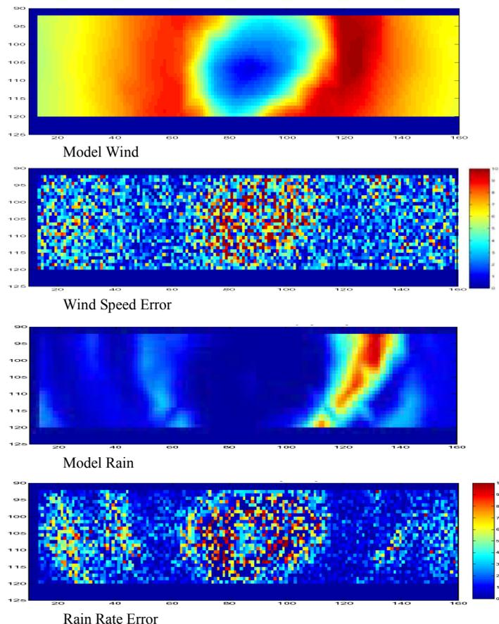
Fig. 5 HIRAD simulated east-West flight leg. Top panel is the modeled wind speed; next is the retrieved wind speed error - color bar is 0-10 knts (5.2 m/s), next is the modeled rain intensity and the bottom panel is the corresponding rain rate retrieval error - color bar is 0-10 mm/hr.
