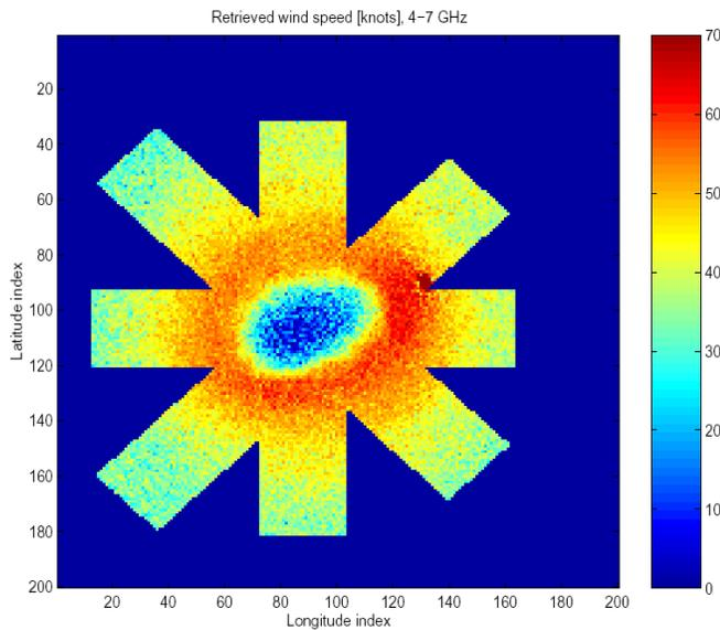
Fig. 2 Simulated HIRad measurements of surface winds from Hurricane Floyd (1999). Ordinate is latitude index ( $0.125^\circ$  steps) and the abscissa is longitude index ( $0.125^\circ$ ). Color scale is 0-70 knts (36 m/s).
