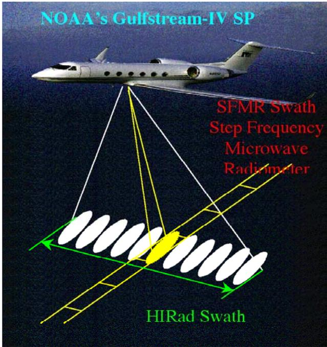
Fig. 1 HIRad measurements from NOAA's hurricane surveillance aircraft.
