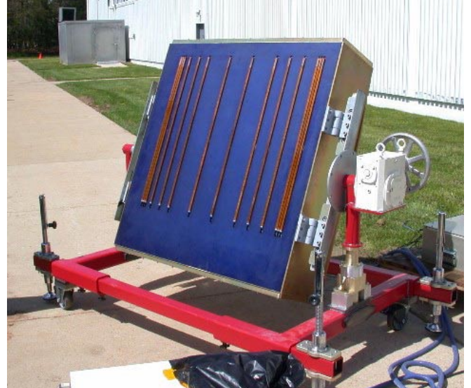
Figure 2. LRR-X deployed at NASA Goddard on 24 April 2003. 14 element thinned linear array of X-Band slotted waveguide antennas (copper) are mounted on an extended ground plane (blue) to reduce backlobes.
