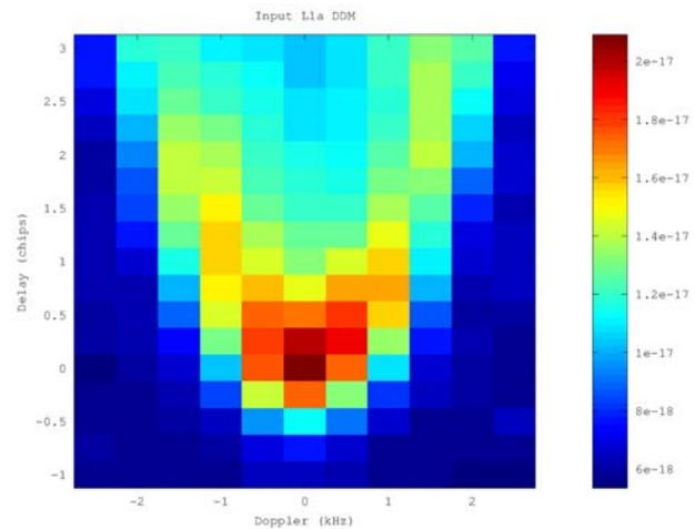
Fig. 3. Simulated Level 1A delay Doppler Map showing signal power in Watts spreading over the surface in both delay and Doppler.
