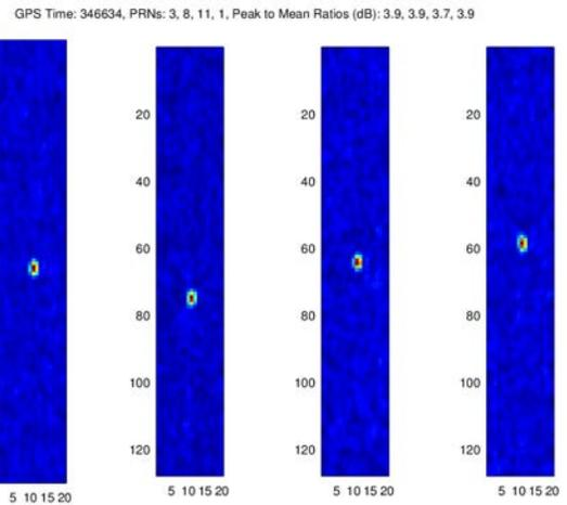
Fig. 5. Example of 4 instrument processed DDMs generated during the 15 minute GSS simulation.
