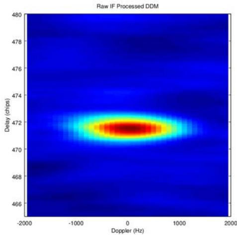
Fig. 4. Delay Doppler map of a direct signal processed in the raw IF data generated by the instrument. DDM is shown in units of uncalibrated counts.
