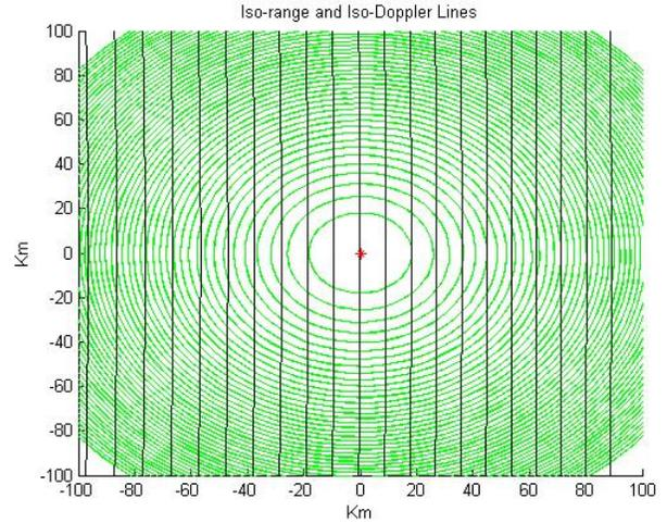
Fig. 2. Example of delay and Doppler spreading over the surface. Lines of constant delay are shown as ellipses while lines of constant Doppler are shown as parabolas (resembling vertical lines in the figure due to the spacecraft geometry).
