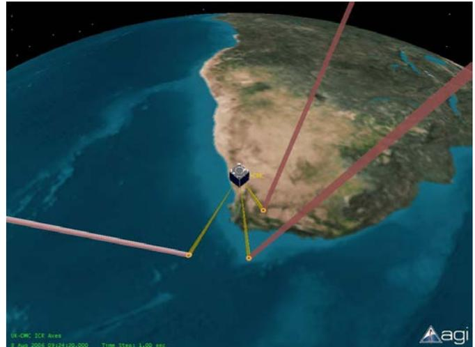
Fig. 1. Illustration of the GNSS reflections remote sensing concept. A single satellite, properly configured, is capable of receiving forward scattered GNSS signals from multiple GNSS satellites, including reflections off the ocean, land and ice surfaces. Figure taken from [14] with permission.
