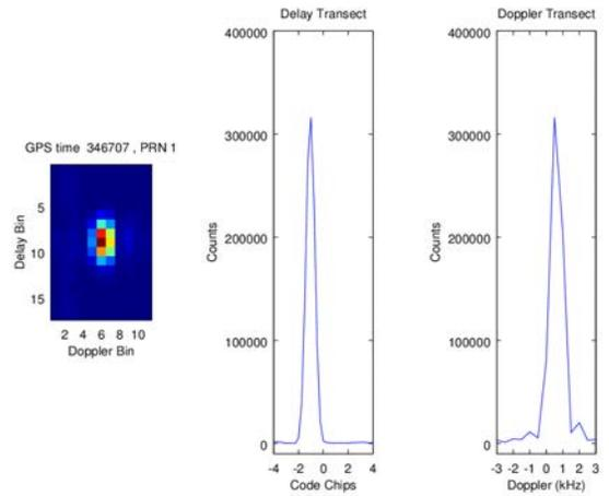
Fig. 6. Example of a single compressed DDM processed by the instrument and the delay and Doppler cuts through the center.
