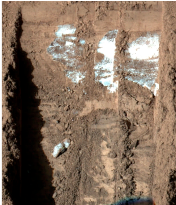
Fig. 1. Image of millimeter-thick clean, soft ice at the bottom of a trench excavated by Phoenix in the Mars Arctic. Note the cylindrical portion of clean ice at the lower left of the trench. In contrast, pore-filling ice found in other trenches was extremely hard [11].
